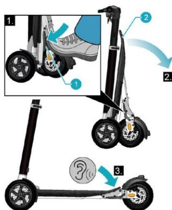
Figure 9: Unfold the folding mechanism
