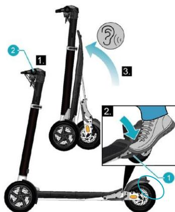
Figure 10: Close the folding mechanism
