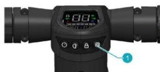
Figure 7: Setting support level
