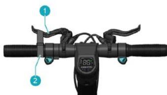
Figure 5: Locking the brake
