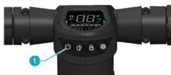
Figure 3: Switch On / Off
